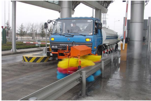
Fig.2. Usage of trucks and big brushes to wash guardrails[3]
